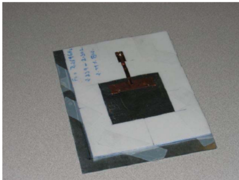
Figure (a): Microstrip Rectangular Patch using Microstrip line feed on Foam substrate
